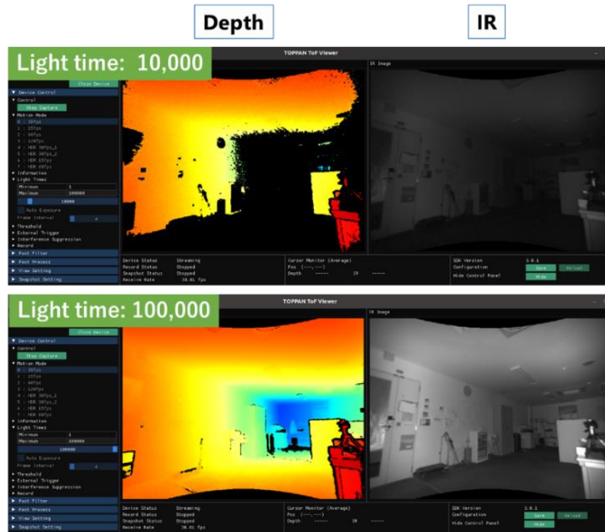
Figure 15. Changing "Light Times" affects depth sensing performance
