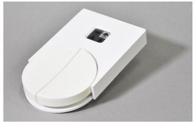
Left: Newly developed electronic paper display. Segmented EPD technology enables ultralow power consumption.
